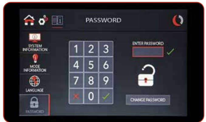
Password protection option maintains integrity of the program database to ensure repeatability.
