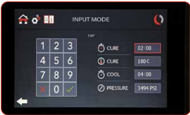
Pop-up keypad makes numerical entry easy. The 7" color LCD touchscreen is used to control all functions and is extremely easy to navigate, allowing greater efficiency among users.
