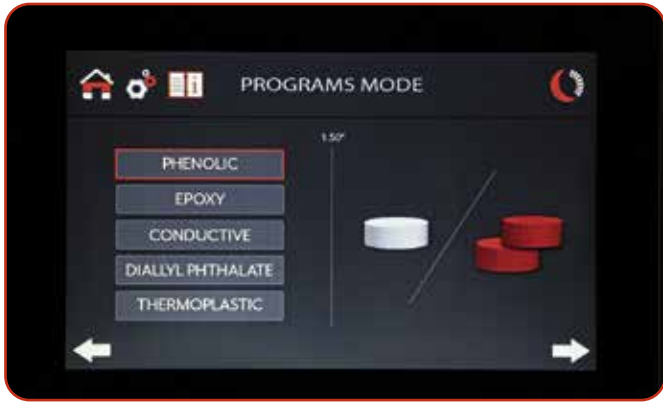
Prepare two mounts per cycle up to 2" / 50 mm.
