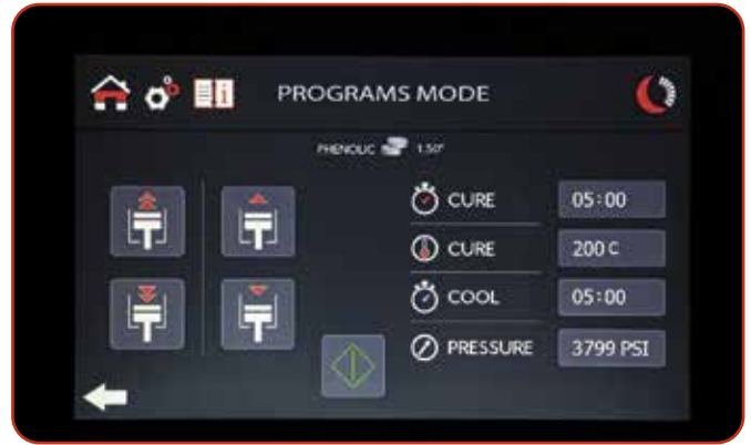
Intuitive, icon-based interface includes option for one-touch or momentary-touch ram extension and retraction.
