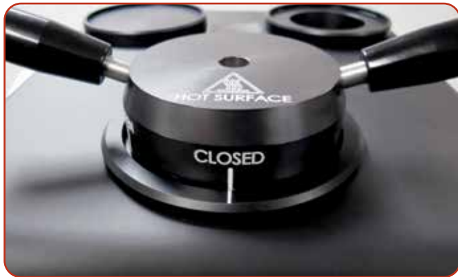
Safety sensor requires full closure of bayonet cap before cycle start.
