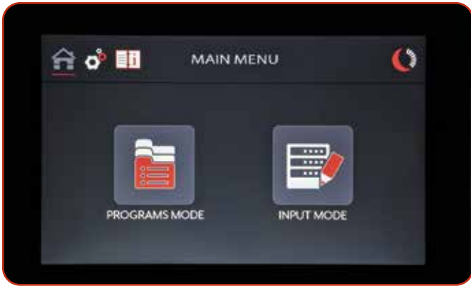
Choose Input Mode when entering data manually, or use Programs Mode to access the pre-loaded database of 80 preset programs that can be changed or customized according to material.
